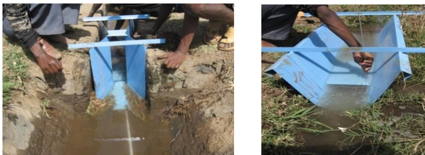
Fig.1. Devices used to measure discharge: cutthroat flume (left) and partial flume (right)
